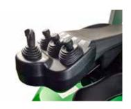
On board the M300H is available with a choice of mechanical or electronic controls
